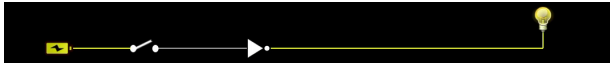
Figure 3: A straw man example of netlist reverse engineering. The goal is to light the bulb which needs a binary input value of 1. Knowing that the logical NOT gate can invert the signal from 0 to 1, we make the switch open (0) to light the bulb.
