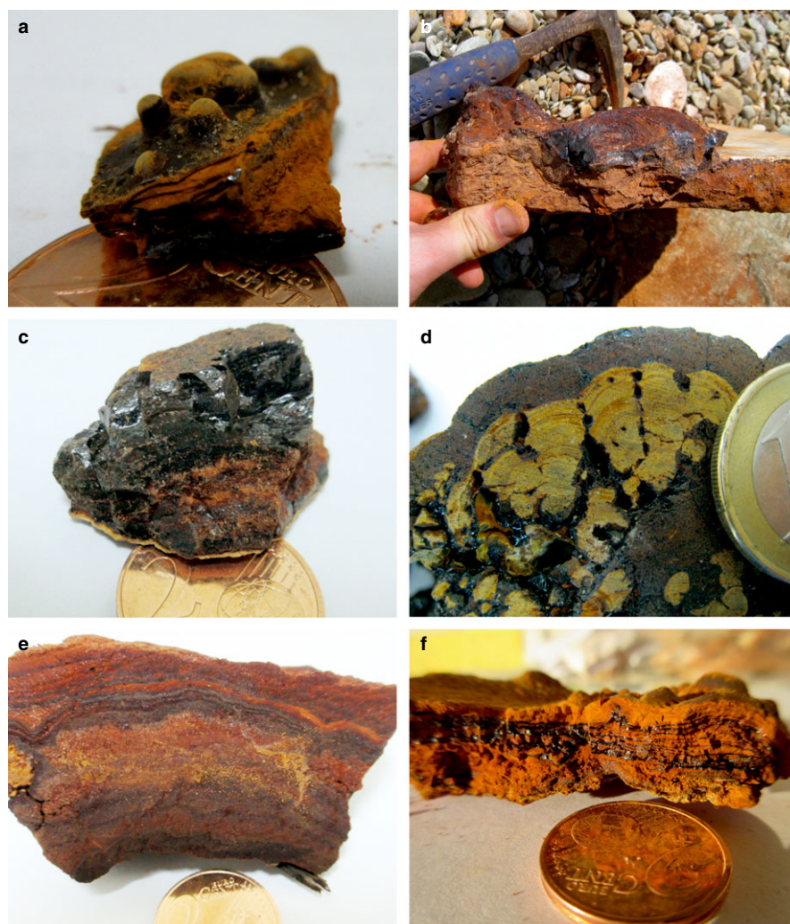
FIGURE 4 Different macro- and microfacies of Ila Fe-rich travertine deposit. (a) Spicular, knob-like Fe-rich thermogenic travertine deposition from inside the borehole (upper part). (b) Dense Fe-rich travertine deposition. (c–f) Fe-rich laminae/bands with varying thickness from few mm up to few cm, alternating with Ca-rich laminae/bands
