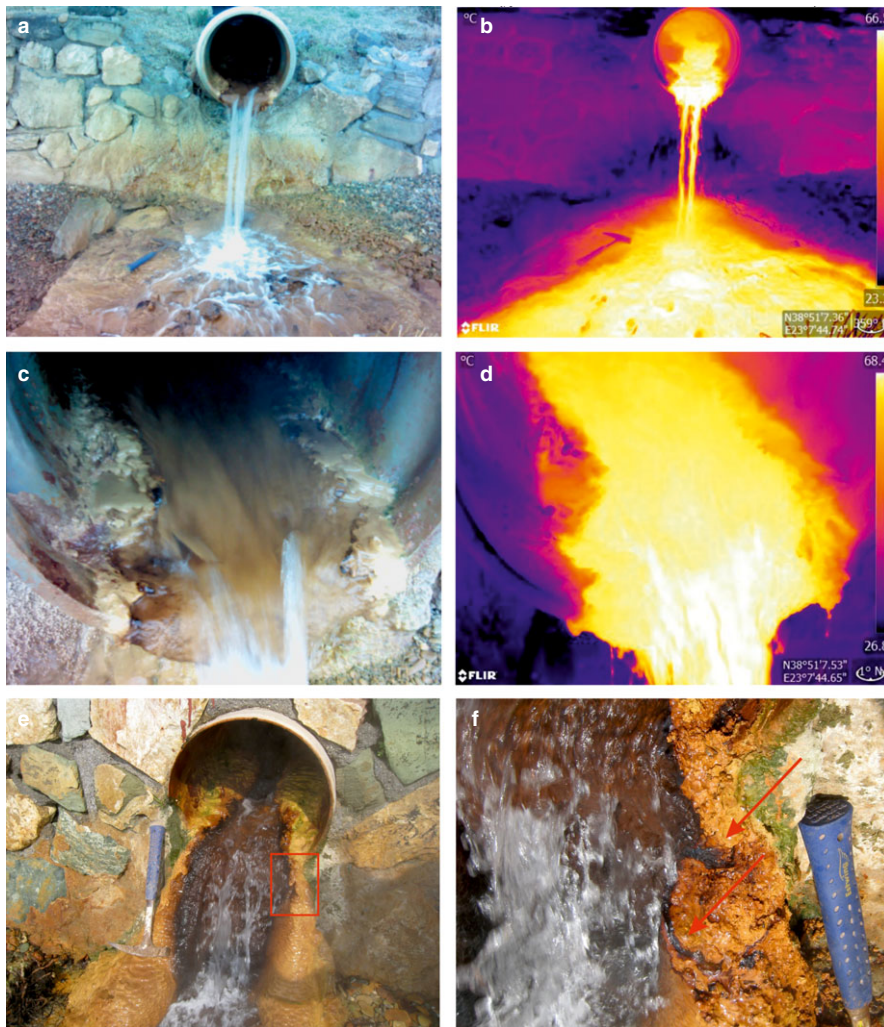
FIGURE 2 Paired views of Ilia's hot spring pictures and corresponding thermal images of the same area. In the right side of each thermal picture, a colour column shows the temperature scale corresponding to the colours. (a and b) General view of the hot water venting out from the pipe. (c and d) Close view of the pipe end point. (e) Venting point of the hot water and associated deposition. Orange-yellowish colour component is Ca-rich and brownish-metallic colour component is Fe-rich. At close-up image (f) could be observed that inside the Ca-rich component are developing Fe-rich bands (see red arrows)
