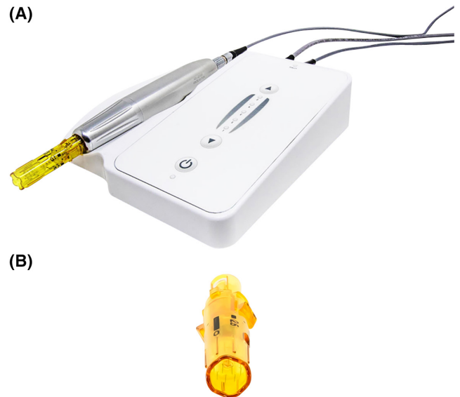
FIGURE 8 (A) Illustration of the DermaPen micro-needling device. (B) Illustration of the DermaPen micro-needling tip. Note that 12 small micro-needles exist in such a device which repeated penetrate within 0.25 to 2.5mm in depth within facial tissues at roughly 3–5000RPMs. Reprinted with permission from Davies/Miron. 8
