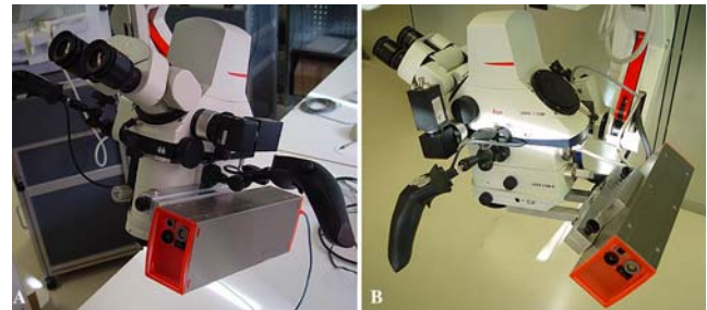
Fig. 1 Two designs for the tracking integration in the surgical microscope. The position of the tracking camera can be changed depending on the working distance needed for the operation and the position of the patient
