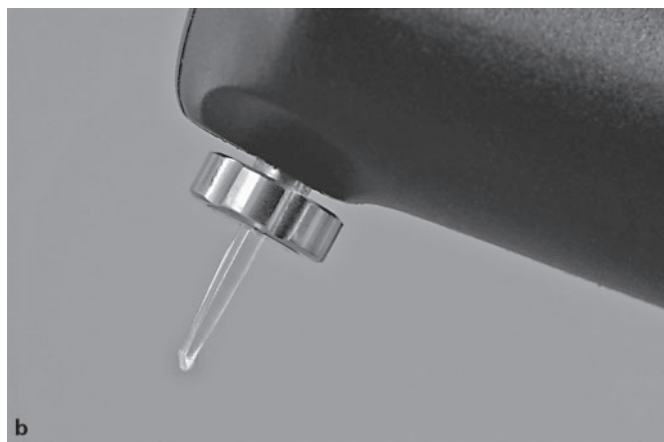
Fig. 1. a LFpen with the tip for measurement of the fluorescence on approximal surfaces. b Close-up of the tip and the knob for turning it around.
