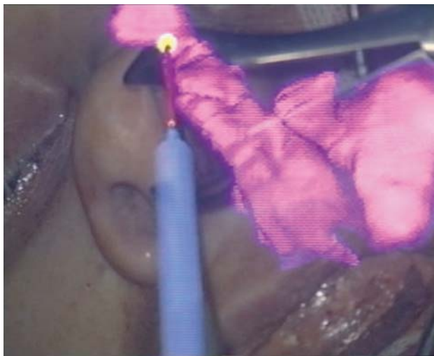
Fig. 15 Interactivity with the augmented reality system. A virtual model of the tool is overlaid to the real tool. Trajectory ( red ) and intersections ( yellow ) are displayed
