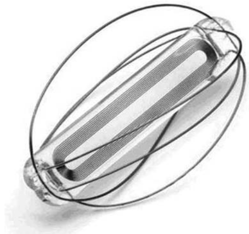
Fig. 1 Implantable EndoSure™ wireless aneurysm pressure sensor measuring 30 \times 5 \times 1.5 mm (CardioMEMS, Atlanta, GA). The sensor contains no batteries or internal power source, but is instead powered by RF energy provided by a proprietary external electronic antenna that is attached to the receiving station (not shown; courtesy of CardioMEMS, Atlanta, GA)
