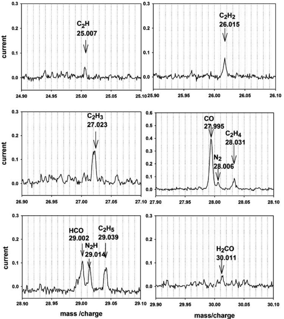
Figure 12. Part of a high resolution background mass spectrum from space at a total pressure of  $4 \times 10^{-11}$  mbar. Integration time was 20 s per mass. The triplets at mass/charge 28 and 29 amu/e can be separated easily.
