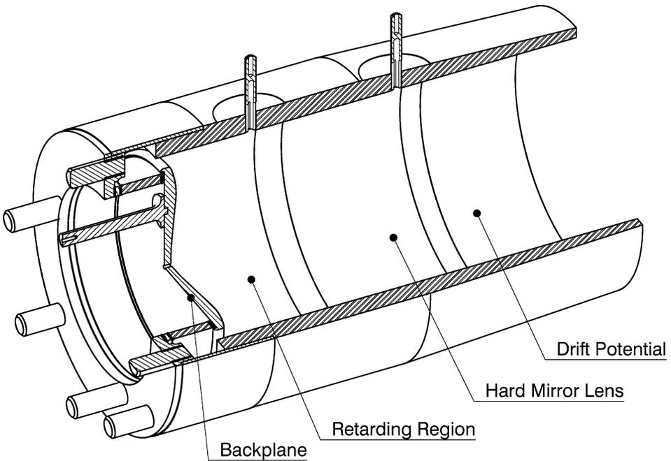
*Figure 18.* The hard mirror structure is based on a ceramic tube body with an inner diameter of 36 mm. Three conductive silver ring electrodes are applied on the inner surface of the ceramic body, with a sophisticated shaped backplane defining the repelling electrical field. The hard mirror contains a conductive outer surface connected to the first inner ring electrode on drift potential to avoid electrical field disturbances affecting ion trajectories passing close by the hard mirror.
