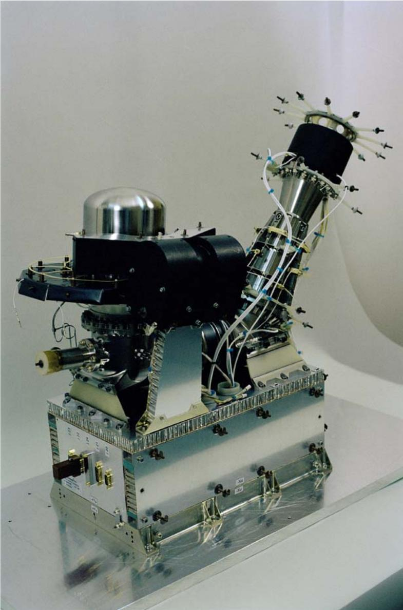
*Figure 5.* Flight model of DFMS without thermal hardware.
