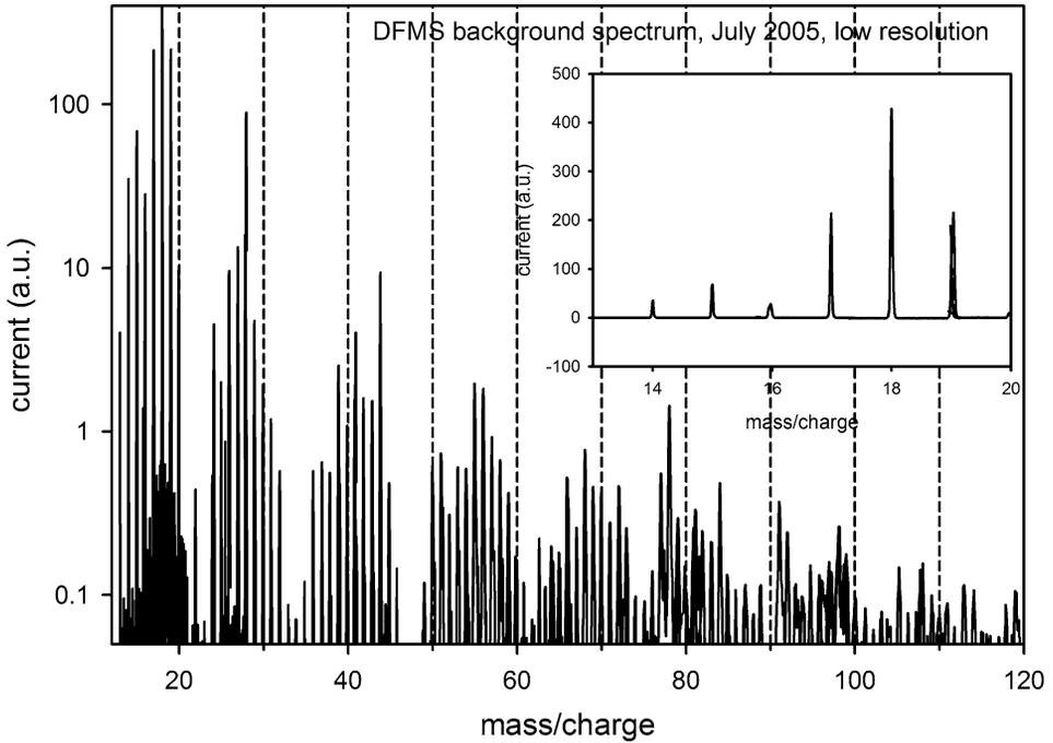
Figure 11. Low resolution background mass spectrum from space at a total pressure of  $4 \times 10^{-11}$  mbar. Integration time was 20 s per mass group. The inset shows the mass range 13–20 amu/e in a linear scale. There is a mass peak on almost all integer mass numbers between 13 and 120 amu/e.
