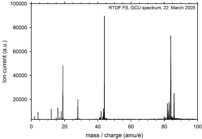
Figure 21. Mass spectrum of the in-flight calibration gas consisting of a mixture of He, CO<sub>2</sub>, and Kr taken in space. Gas pressure in the source was  $1 \times 10^{-9}$  mbar, integration time 200 s.
