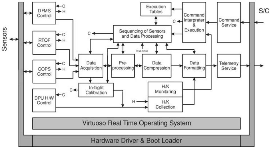
Figure 31. Schematics of the DPU layer model.
