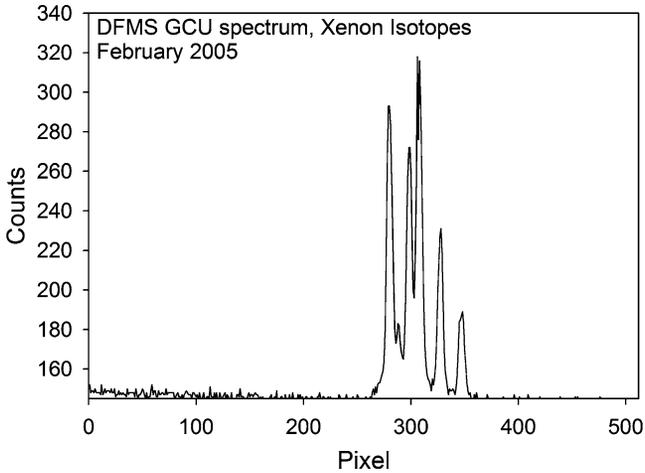
Figure 13. Part of an in-flight calibration mass spectrum from space at a total pressure of  $5 \times 10^{-7}$  mbar test gas. Shown are the Xenon isotopes in low resolution. Integration time was 20 s.
