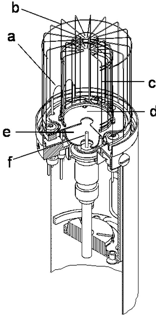
Figure 24. Drawing of the COPS nude gauge showing important components: (a) two filaments, 28 V, (b) outer grid,  $-12$  V, (c) inner grid, 180 V, (d) base plate, 0 V, (e) reflector, 110 V, (f) ion collector.
