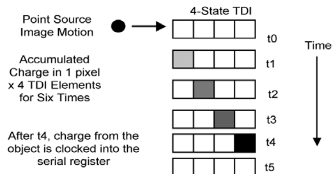
Figure 6. Illustration of 4-line Time Delay and Integration (TDI). HiRISE can use 8, 32, 64, or 128 TDI lines.
