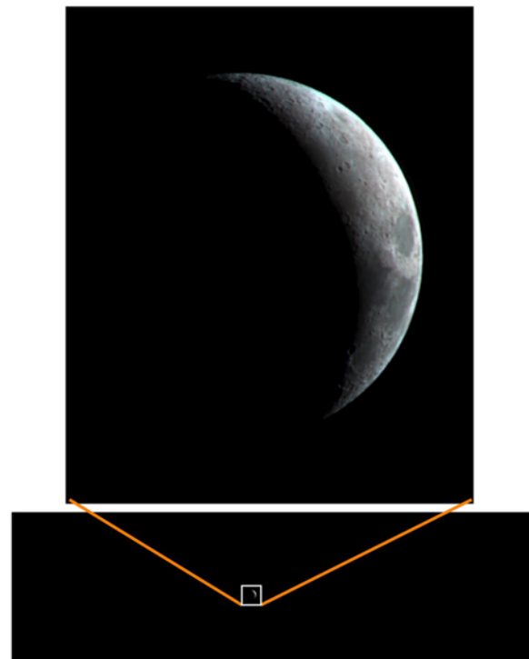
Figure 14. HiRISE image of the Moon acquired 8 September 2005. The bottom image shows the entire red-filter image with 10 CCDs. Image size is 20,048 \times 8,000 pixels. At top is a blowup of the lunar image in color, 10 km/pixel. The color variations are lightly enhanced via use of color ratios. Shown is the nearside at \sim 120^\circ phase angle; Mare Crisium is the dark circular region near right center.
