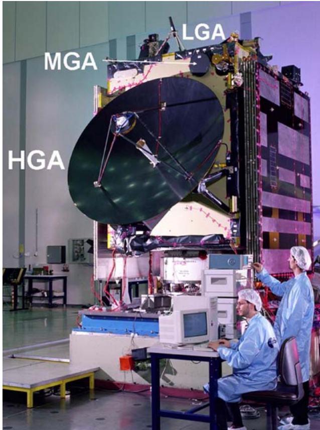
Figure 6. The antenna systems of the Rosetta spacecraft: the High Gain Antenna (HGA) is a parabolic dish of 2.20 m diameter and used as the primary antenna for RSI. Furthermore there are two Medium gain Antennas (MGA) side by side for separate X-band and S-band transmissions and two Low Gain Antennas (LGA, one at the rear and one at the front) for near Earth communications and emergencies.
