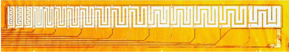
Figure 3. A new type of thermal sensor has been developed by the MUPUS team. A 20\ \mu\text{m} thin layer of titanium on a Kapton substrate is used to measure the temperature (electrical resistance is proportional to the temperature). The same titanium cell can be actively heated in order to perform thermal diffusivity and conductivity measurements (upper panel). 16 such cells and all required electrical connections (thin lines) are laser-sputtered on one Kapton sheet (lower panel). The cell dimensions grow from top (left in image) to bottom. The Kapton sheet is rolled and glued to the inner tube wall of MUPUS PEN.
