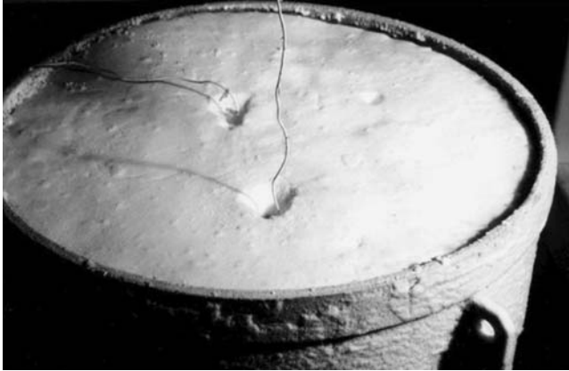
Figure 10. Example of an anchor test shot. The target sample is a sintered CO 2 ice crust with softer material underneath. The shot holes and the anchor cables are visible.
