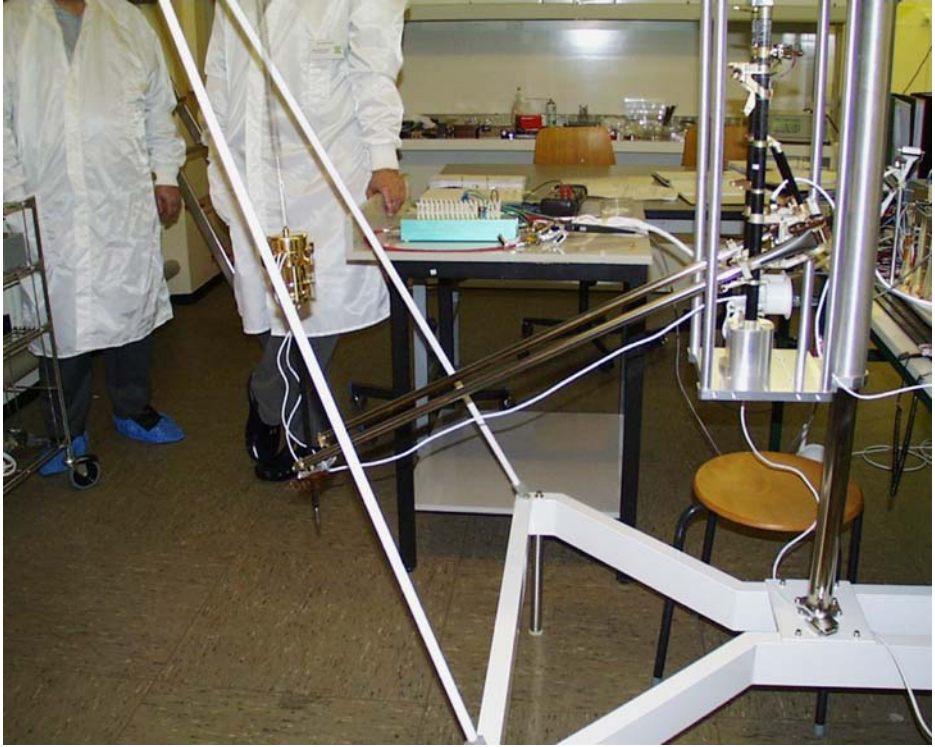
Figure 7. The MUPUS PEN and deployment device during a deployment test.
