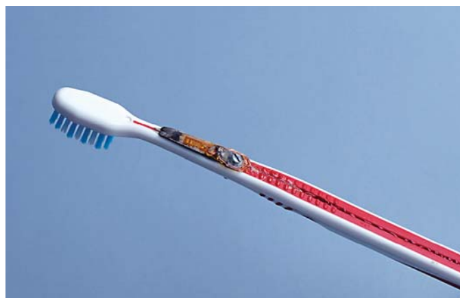
Fig. 1. Toothbrush design. The head of the toothbrush is changeable. Two strain gauges are attached on the upper and lower side of the metallic flap for measuring toothbrushing forces.
