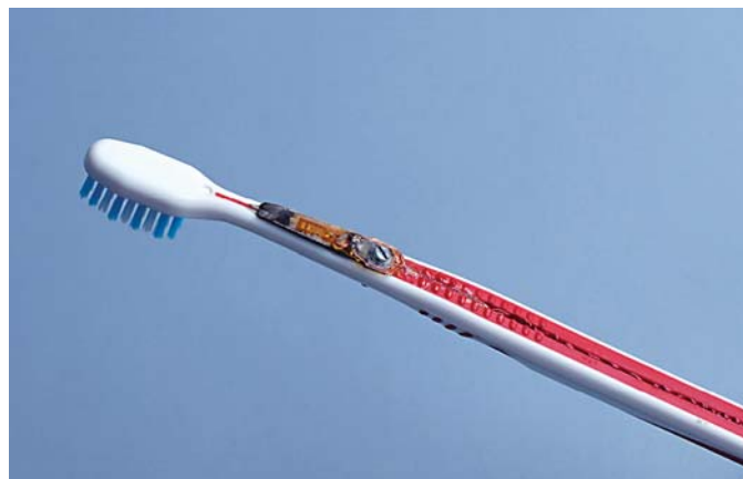
Fig. 1. Toothbrush design. The head of the toothbrush is changeable. Two strain gauges are attached on the upper and lower side of the metallic flap for measuring toothbrushing forces.
