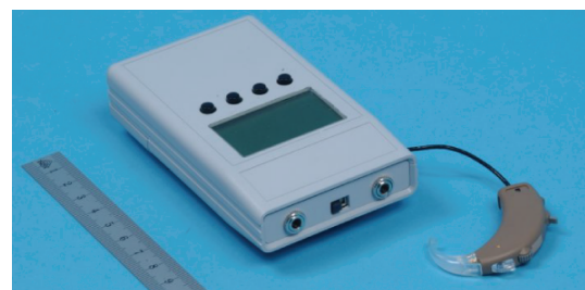
FIGURE 10: Photograph of the portable prototype real-time noise reduction system.
