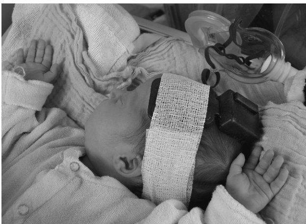
Fig. 2. Wireless NIRI instrument. The advantage of wireless technology is that it is more comfortable and less susceptible to movement artifacts, because there is no cable, which pulls the sensor. The device only weighs 40 g and the battery lasts for approximately 3 h.
