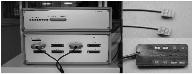
Fig. 1. Left: MCPII measuring system (bottom) and stimulation unit (top). Right: LEDs for visual stimulation (top right). The sensor contains 4 light sources (each with 730 nm and 830 nm LEDs) and 4 detectors (photodiodes), covering an area of 2.5 by 3.75 cm with 10 light bundles (bottom right).
