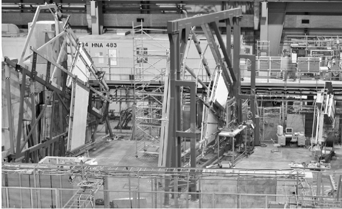
Fig. 2. Picture of the end-cap test stand with six MDT chambers and two TGC stations, taken in July 2003. From left to right: EOL, EML, and EIL MDT chambers; the TGC doublets are close to the middle MDT station.
