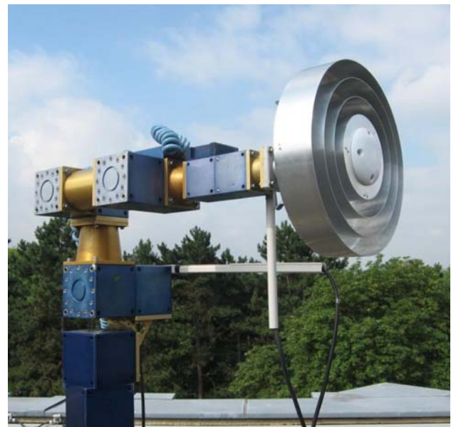
Fig. 2 The IfE robotic measurement system for the automated absolute field calibration with the CHAMP/GRACE/TerraSar-X GPS antenna
