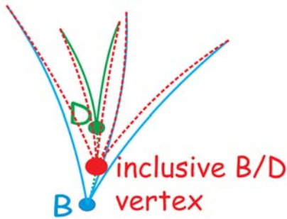
Figure 3: BTagVrtSec fits all displaced tracks to an inclusive vertex.
