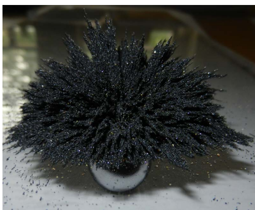
Figure 1. A sample of black magnetic sand from Ladispoli under the action of the magnetic field produced by a spherical permanent magnet located underneath.
