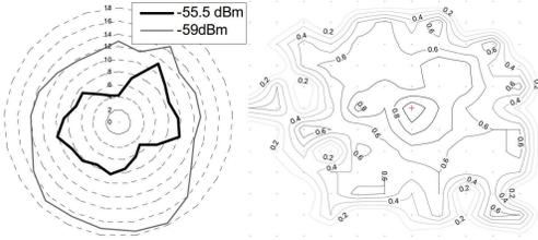
Fig. 1. Irregular radio range(left) and resultant PDR distribution(right)
