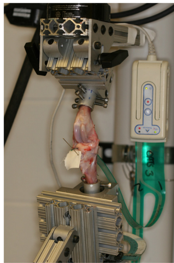
Figure 1 Illustration of the testing apparatus including stifle jig mounted in the material testing machine and digital pressure sensor positioned subadjacent to lateral meniscus.
