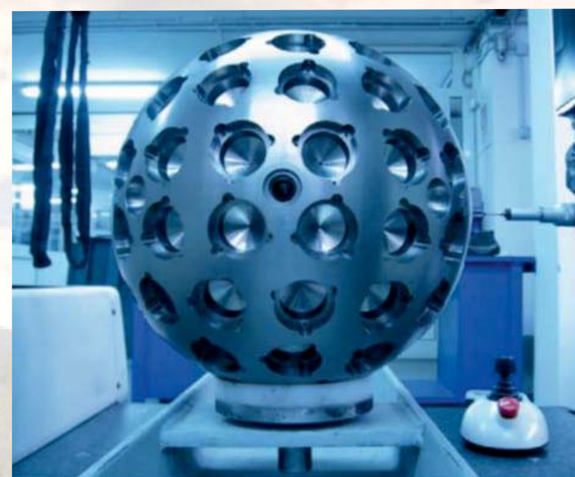
Fig. 1: LARES before embedding the corner cube retro-reflectors (courtesy of ASI)
