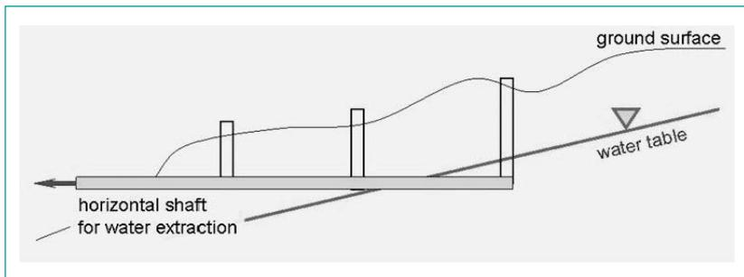
Description of a *qanat* system: Vertical shafts called mother wells (up to 50 metres deep) are dug close to underground springs or water table. Further, several and at more or less regular intervals "ventilation shafts" are dug in a straight line to target (Safriel and Adeel, 2005).
