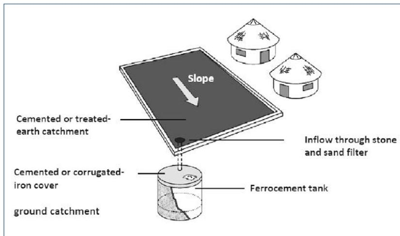
Courtyard catchment system including cemented ground (a road could equally act as a catchment), an underground ferro-cement tank with a cemented, corrugated iron or tiled cover (UNEP IETC, 1998 in Clements et al., 2011).
