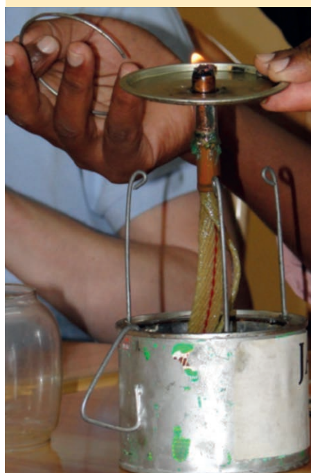
Figure 1: A jatropha oil lamp made from a recycled can in Arusha, Tanzania. A copper tube is added around the wick to conduct heat from the flame to the reservoir. Preheating the oil reduces its viscosity and improves capillary action along the wick. Deposits of soot on the wick necessitate frequent cleaning or cutting. (©Ehrensperger)
