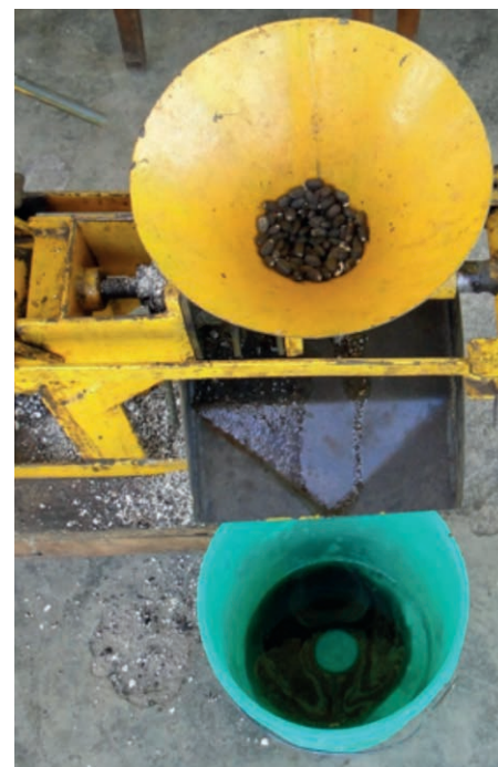
Figure 3: A ram press fixed on a wooden beam in Arusha, Tanzania. Seeds are placed in the yellow funnel; the resulting oil flows over an iron plate into a bucket below. Extraction of the oil is slow and tedious, and it requires filtering after extraction. (©Ehrensperger)
