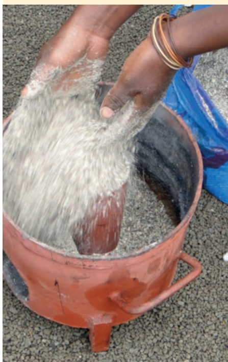
Figure 2: Jatropha press cake being poured into an experimental cooking stove in Arusha, Tanzania. The central cylinder is removed after filling the stove, and the fire is lit within the hollow tube. Smoke is given off during combustion because the press cake contains oil residues, especially following pressing with low efficiency ram presses. (©Ehrensperger)
