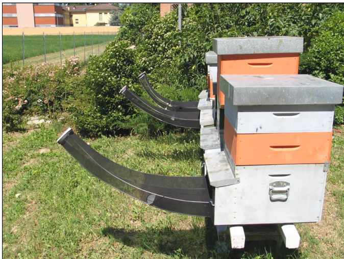
Fig. 5. Bologna Traps, without collection containers, attached to the entrance of honey bee colonies.
