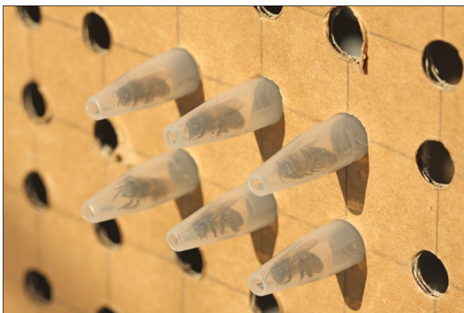
Fig. 17. Isolation cages created by drilling 2-3 mm ventilation holes in the tip of 1.5-ml microcentrifuge tubes. Cages and storing device courtesy of Ulrike Hartmann, Swiss Bee Research Centre.
