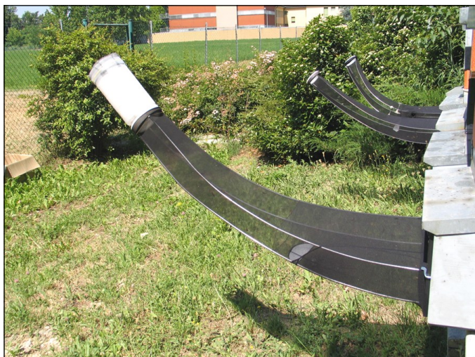
Fig. 8. A Bologna Trap with a ventilated collection container installed on the foreground colony to obtain exiting honey bees.
