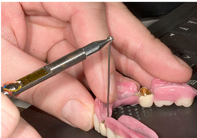
Fig. 1 Measuring stylus with strain gauge (arrow) fixed to the flat surface, measurement of the retention force by aligning the flat surface of the strain gauge on the measuring stylus at right angles to the withdrawal direction of the wire retention
