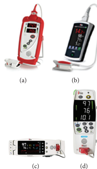
FIGURE 1: Handheld spot check devices, (a) Pronto; (b) Pronto-7, and continuous monitoring bedside devices, (c) Radical-7 and, (d) Rad-87.
