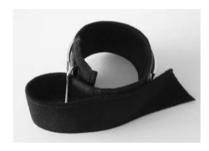
${f Fig.~3}$  Cuff that connects the rotary module with the human upper arm
