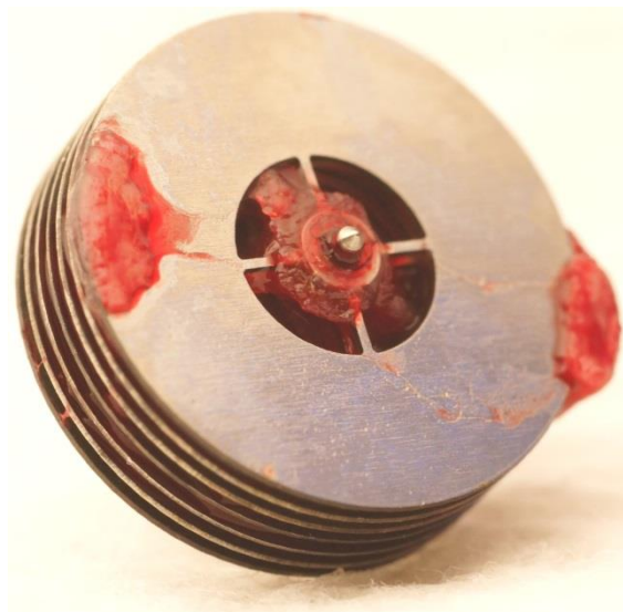
Figure 4. Observation of thrombi on the rotor
