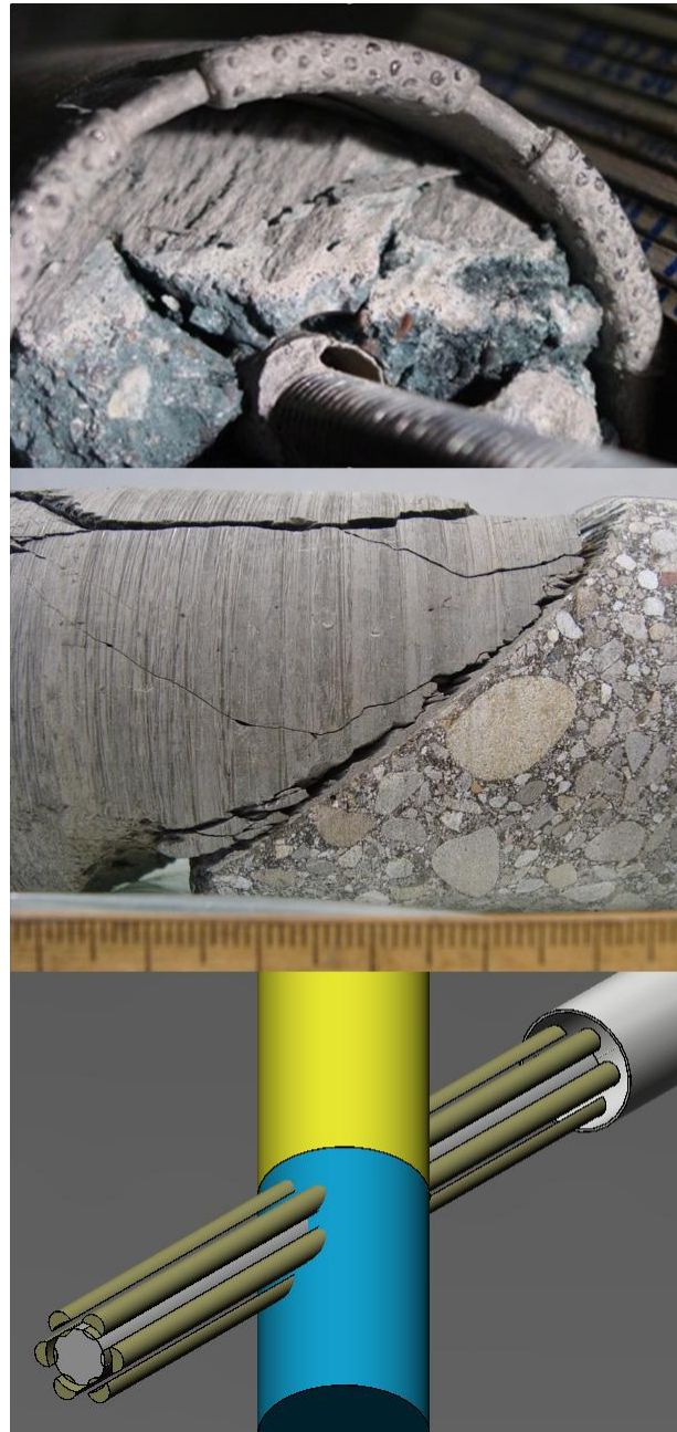
Fig. 2 Example of drilling technique used in 2009 with a single re-forcement glued in prior to overcoring (upper images, outer diameter of drillbit = 86 mm). Shown is a sample of LAC with white reaction zone at interface, and a thin layer of Opalinus Clay preserved at the interface (top), and OPC (sealing plug) mechanically separated from Opalinus Clay (middle). Schematic of optimised stabilisation technique used in 2012 (lower image, see text for explanation).
