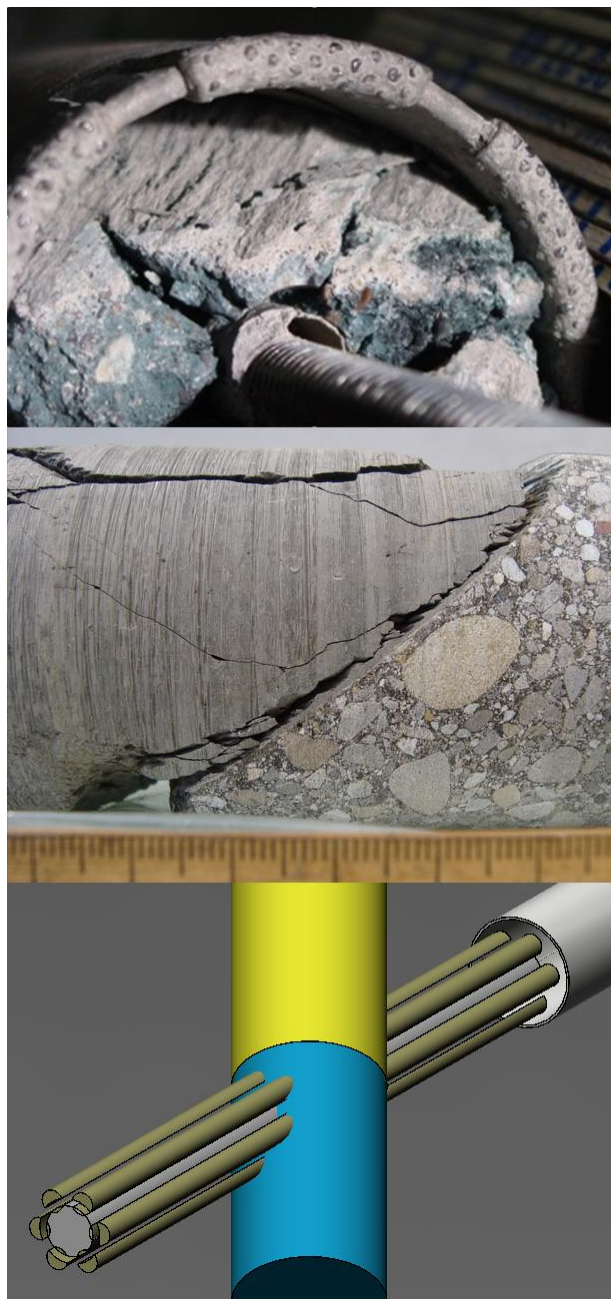
Fig. 2 Example of drilling technique used in 2009 with a single re-enforcement glued in prior to overcoring (upper images, outer diameter of drillbit = 86 mm). Shown is a sample of LAC with white reaction zone at interface, and a thin layer of Opalinus Clay preserved at the interface (top), and OPC (sealing plug) mechanically separated from Opalinus Clay (middle). Schematic of optimised stabilisation technique used in 2012 (lower image, see text for explanation).
