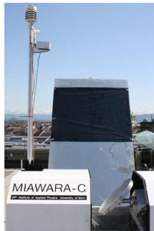
Figure 4. Picture of the test setup for the emissivity measurements using MIAWARA-C radiometer. The MLI sample covers the Aluminum reference reflector about 50% of the measurement time. A weather station is installed nearby the instrument (left).
