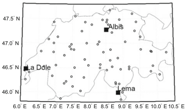
Figure 2: A map of Switzerland showing the locations of the 70 rain gauge stations of the MeteoSwiss surface meteorological network (ANETZ, are indicated by open circles). The three C-band Doppler precipitation radars of MeteoSwiss used in this study are located on mountain tops, near Zurich on Albis (925 m above sea level (ASL)), near Geneva on La Dôle (1675 m ASL), and near Lugano on Monte Lema (1625 m ASL) are depicted by filled squares.
