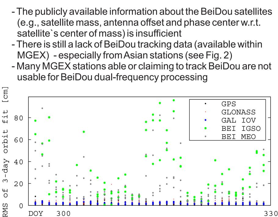
Fig. 7: RMS of 3-day longarc fit of CODE MGEX orbits (GPS, GLONASS, Galileo, BeiDou) for the time interval DOY 13/300 - 13/330
