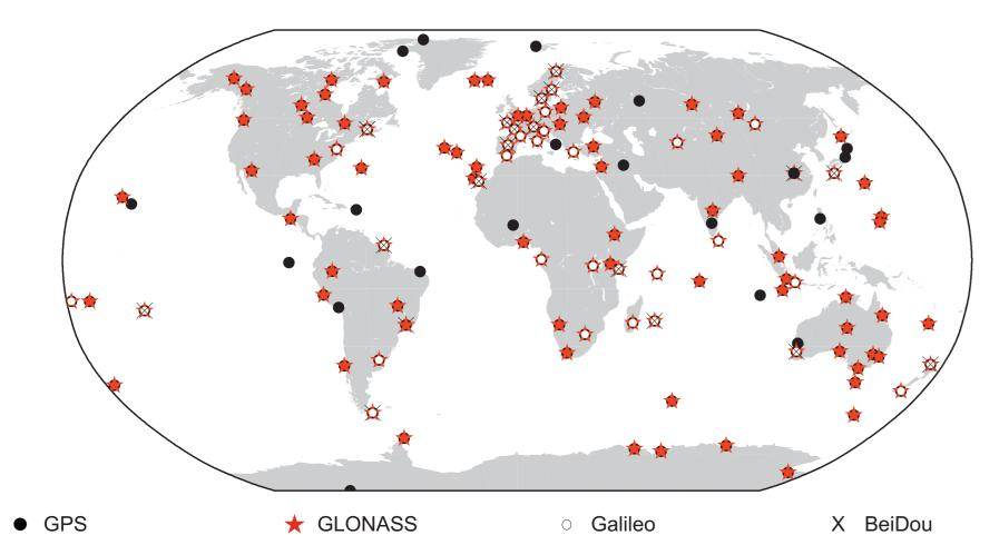
Fig. 2: Tracking network as used for the generation of the CODE MGEX solutions (status DOY 13/300).
