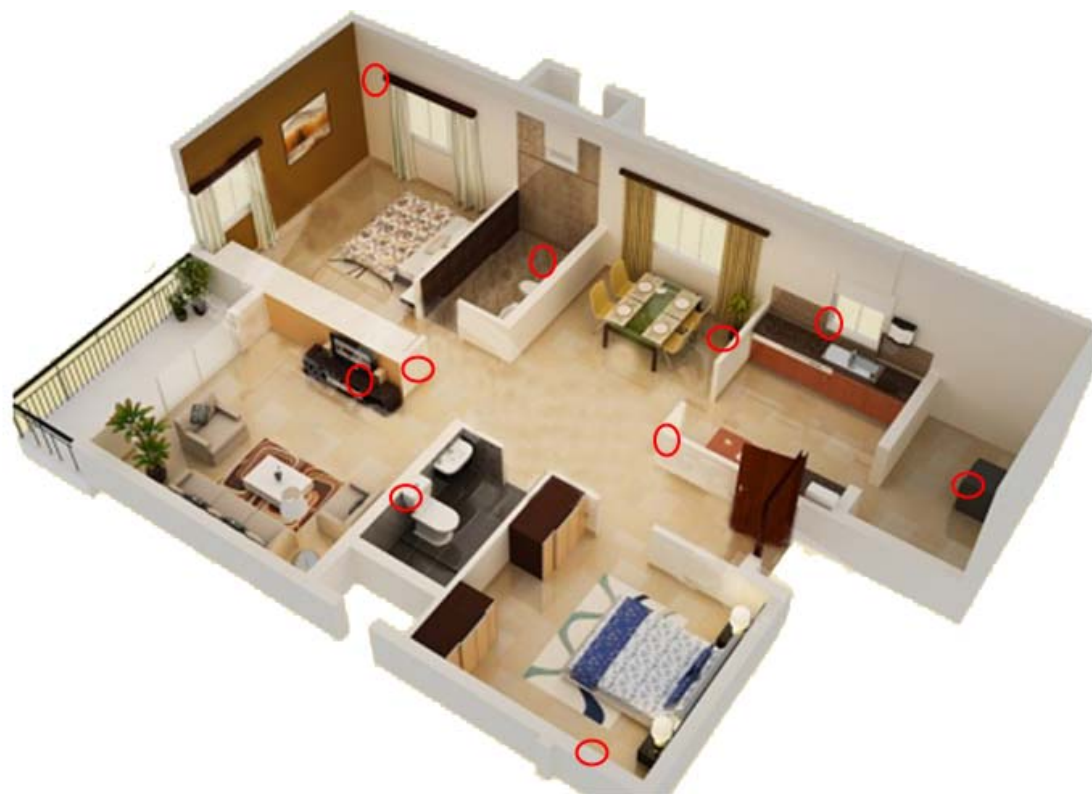
Example setup installed in a 2-bedroom apartment (sensor boxes indicated with red circles).
