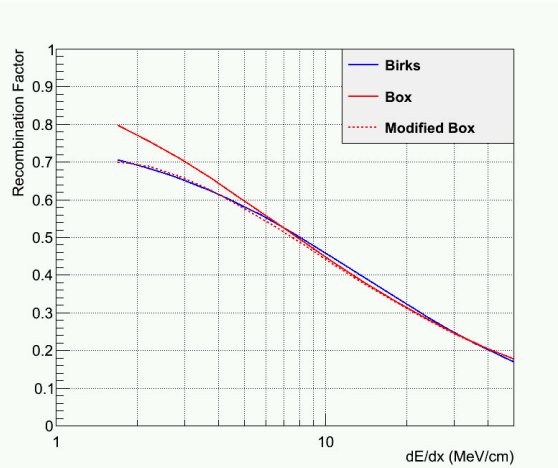
Figure 1. Qualitative comparison of the recombination factor for the Birks equation using ICARUS parameters (blue curve), the ‘‘canonical’’ Box model with \alpha = 1 and \beta = 0.30 (red curve) and a ‘‘modified Box’’ equation with \alpha = 0.93 and \beta = 0.30 cm/MeV (dotted red curve).
