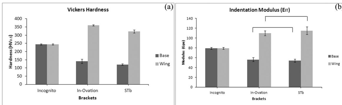
**Figure 4** Graphs showing the Vickers hardness (a) and indentation modulus (b) for all brackets tested. The same mean values and standard deviations were appended to Incognito for base and wing regions as it is a one-piece structure. Connecting lines imply mean values without statistical significant differences ( $P > 0.05$ ).
