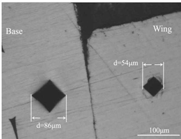
**Figure 2** Cross-section image illustrating indentation impression on softer base and harder wing alloys. The interface between the two parts is also readily shown in the middle (Bar 100  $\mu\text{m}$ ).
