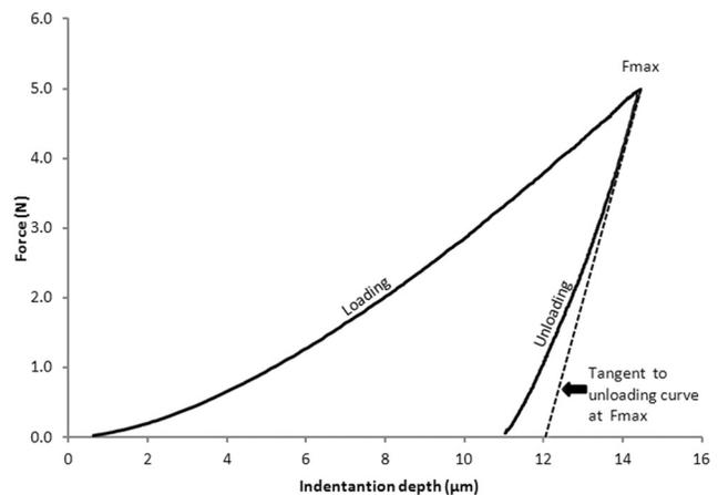
**Figure 3** Representative curve of a force-indentation depth of brackets tested with loading–unloading cycle. Tangent to unloading curve at maximum force ( $F_{\text{max}}$ ) is also shown with dotted line.
