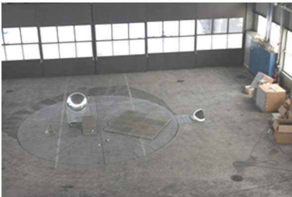
Fig. 12 Test scene for active noise illumination. Metal box and absorbers on the platforms, diffuser box and source on the right
