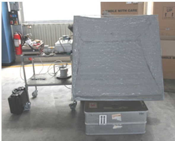
Fig. 4 High power noise source (left) coupled with large size diffuser box (right)
