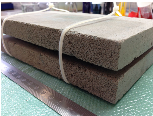
Fig. 2 Ceramic foam plates bound together by standard plastic cable ties
