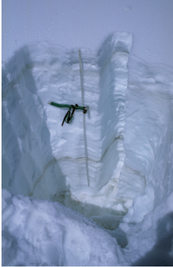
FIGURE 2: Photograph of snow pit 2 of 15.06.2006. Clearly visible are the prominent dust layers.
