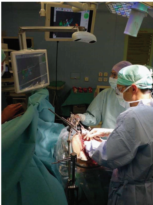
Figure 2 CAScination navigation system as it is placed at the head end of the patient with the sterile-covered touch screen facing towards the surgical team. This allows for easy access and constant interaction with the 3D planning model displayed on the screen.
