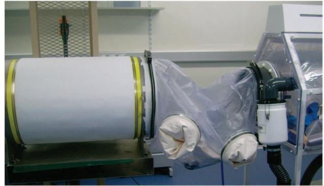
**Figure 2** Sterile connection between a material drum and a flexible film isolator. The large steel drum contains sterile materials to be imported into the isolator, such as food, bedding, or cages. The drum is sealed and autoclaved and then connected to the isolator via a plastic sleeve that is sterilised by spraying with 2% peracetic acid, which then permits transfer of the sterile material into the isolator.
