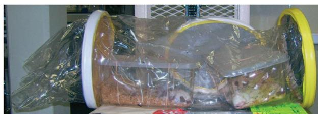
**Figure 4** Specialised transport sleeve. The photo shows an example of a specialised transport sleeve developed to allow shipping of germ-free animals between facilities. The example shown is available from Taconic. Many germ-free facilities have developed their own transport devices that reflect the design of their isolators. Such transport containers allow importation of germ-free or isobiotic mice into isolators at the new facility and ensure hygiene is maintained during transport.
