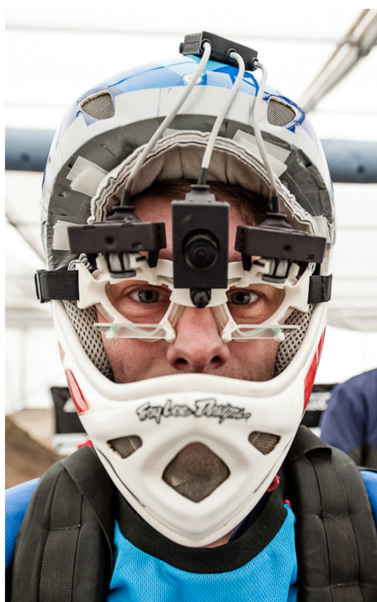
Figure 2: A mountain biker wearing a state-of-the-art third party eye-tracker which is not appropriate for sports
