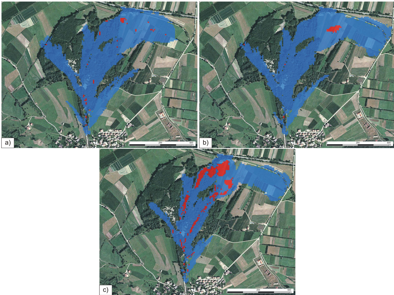
Fig. 15. Variations in flow depth and extent of a design event with a return period of 30 years (actual climate conditions) using different input parameters for the critical shear stress. (a) Flow depths for a design event with a return period of 30 years (scenario 2000). Critical shear stress parameter of 200 Pa. (b) Flow depths for a design event with a return period of 30 years (scenario 2000). Critical shear stress parameter of 400 Pa. (c) Flow depths for a design event with a return period of 30 years (scenario 2000). Critical shear stress parameter of 800 Pa.
