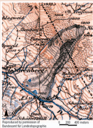
FIGURE 2 1918 topographic map, showing the open scars on either side of the mass and the typical accumulation features developed in 1910 and 1912. The few houses with the church (at the center of the village) are located in a safe place. (Map reproduced by permission of Bundesamt für Landestopographie, BA024084)
