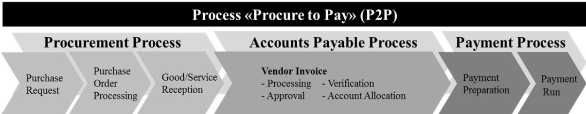
Figure 11: SBB’s P2P Process (SBB 2011)
