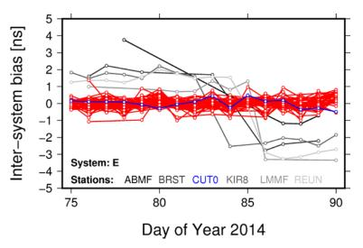
6 stations equipped with TRIMBLE NETR9 with same firmware upgrade from version 4.80 to 4.85.
