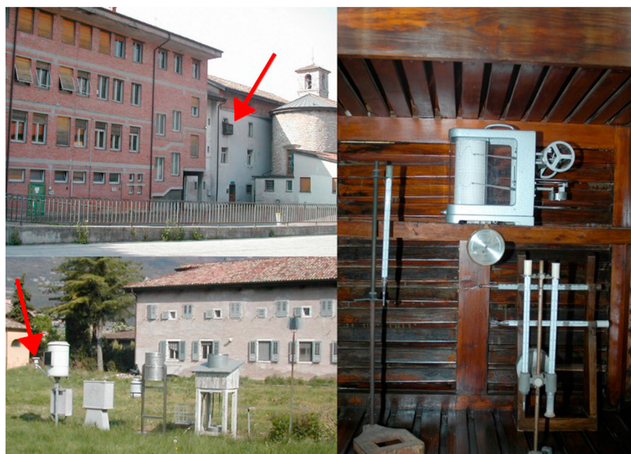
Figure 2. Pictures of the meteorological observatory of Rovereto taken around 2003: (top) the meteorological window and its surroundings, (bottom) the automatic weather station (arrow indicates the thermometer), and (right) the inside of the meteorological window.
