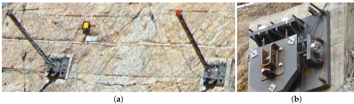
Figure 7. Post base measurement system (a) with installed posts at a test site and (b) in detail showing three pressure sensors orthogonal to the rock face and three two-way sensor installations parallel to the rock face (source: Igor Paramassi S.p.a.).
