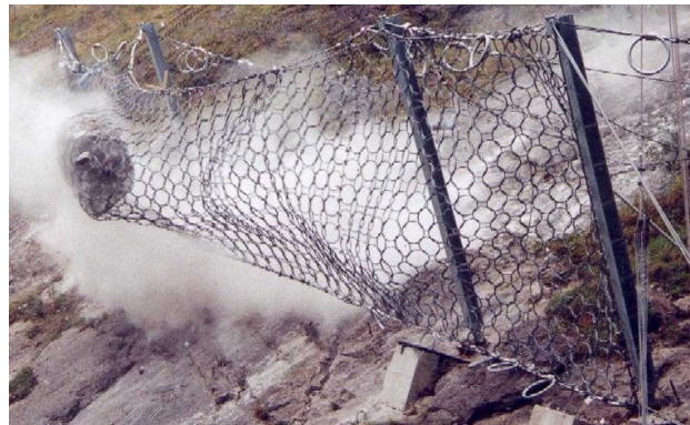
Figure 1. Example of flexible rockfall protection barrier in action (source: Fatzer).
