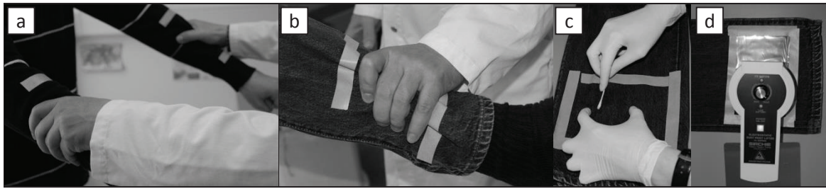
335 Figure 2 Simulated aggression. Victims carrying a cotton sweater and a pair of jeans were thoroughly touched at their a) 336 forearms and b) ankles. The areas were subsequently limited to 10x15cm and sampled either by c) wet cotton swab or d) 337 electrostatic dust print lifter (DPL).
