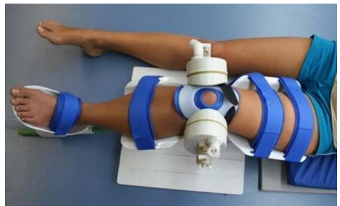
Fig. 1 Custom-made loading device, with footplate, for generation of a compressive force (50% of body weight) on the knee joint
